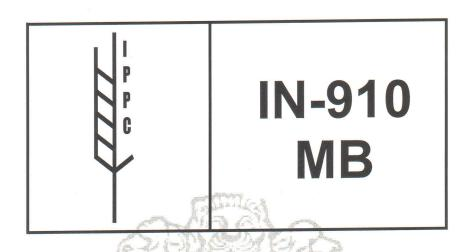
**Note:** Markings should be according to the model shown above (12 x 6 cm), legible, permanent, not transferable, placed in a visible location and preferably marked by a stencil with black ink. The letter size should be a minimum of 2.5 cm. Recycled, remanufactured or repaired wood packaging material should be re-certified and re-marked. All components of such material should have been treated.
